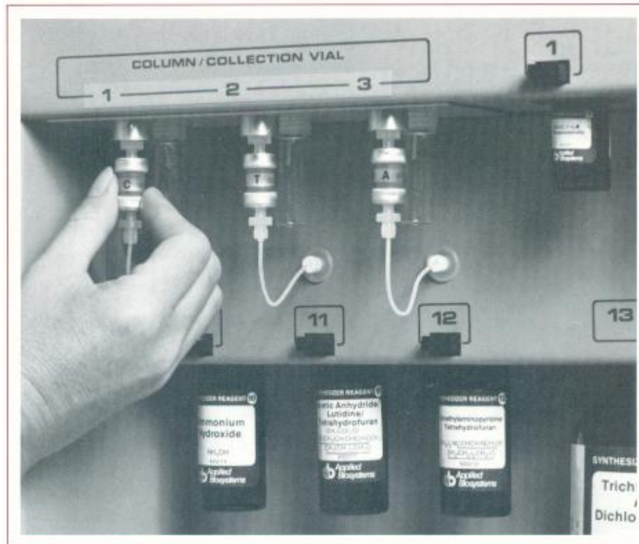
Three columns for simultaneous synthesis of oligonucleotides.
