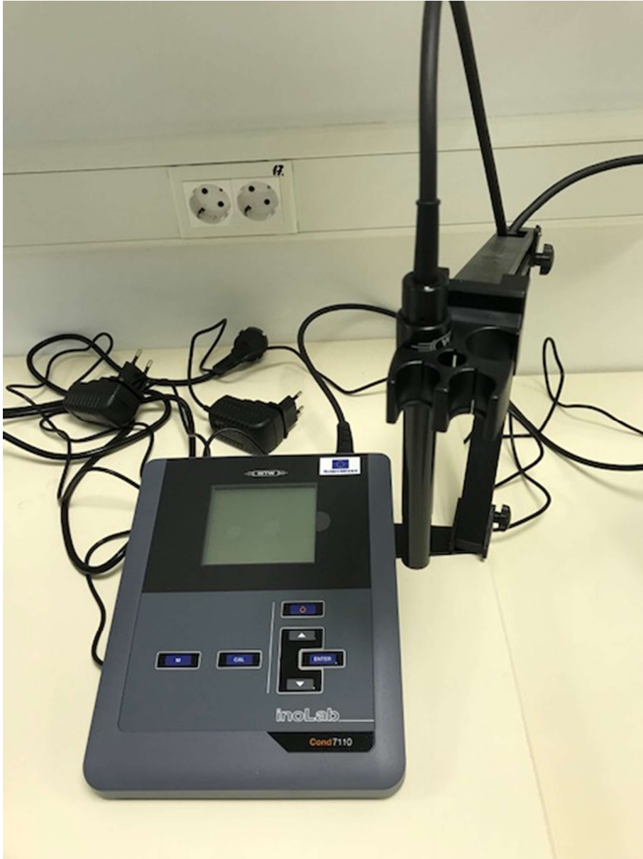
Konduktometar, model: Conductivity benchtop meter inoLab® Cond 7110
