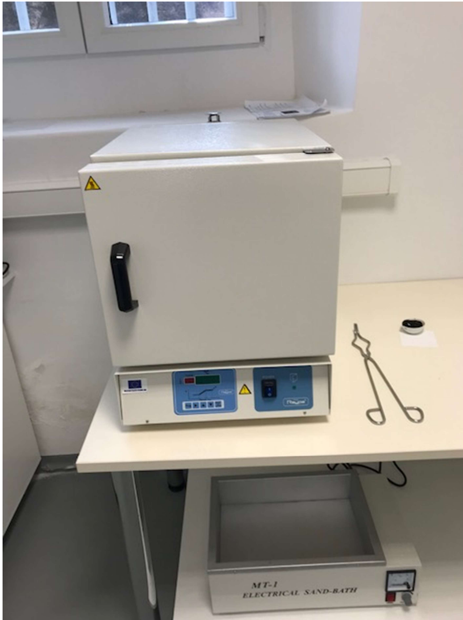
Mufoľna peć, model: HM – 2 MP
