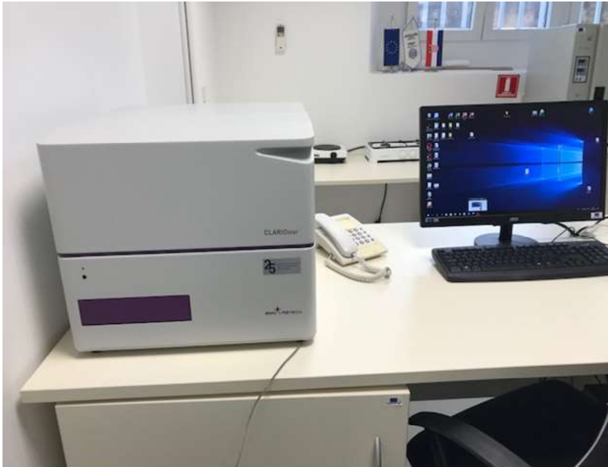
Spektrofluorimeter Clariostar, BMG LABTECH, Offenburg, Germany Spektrofluorimeter Clariostar, BMG LABTECH, Offenburg, Germany
