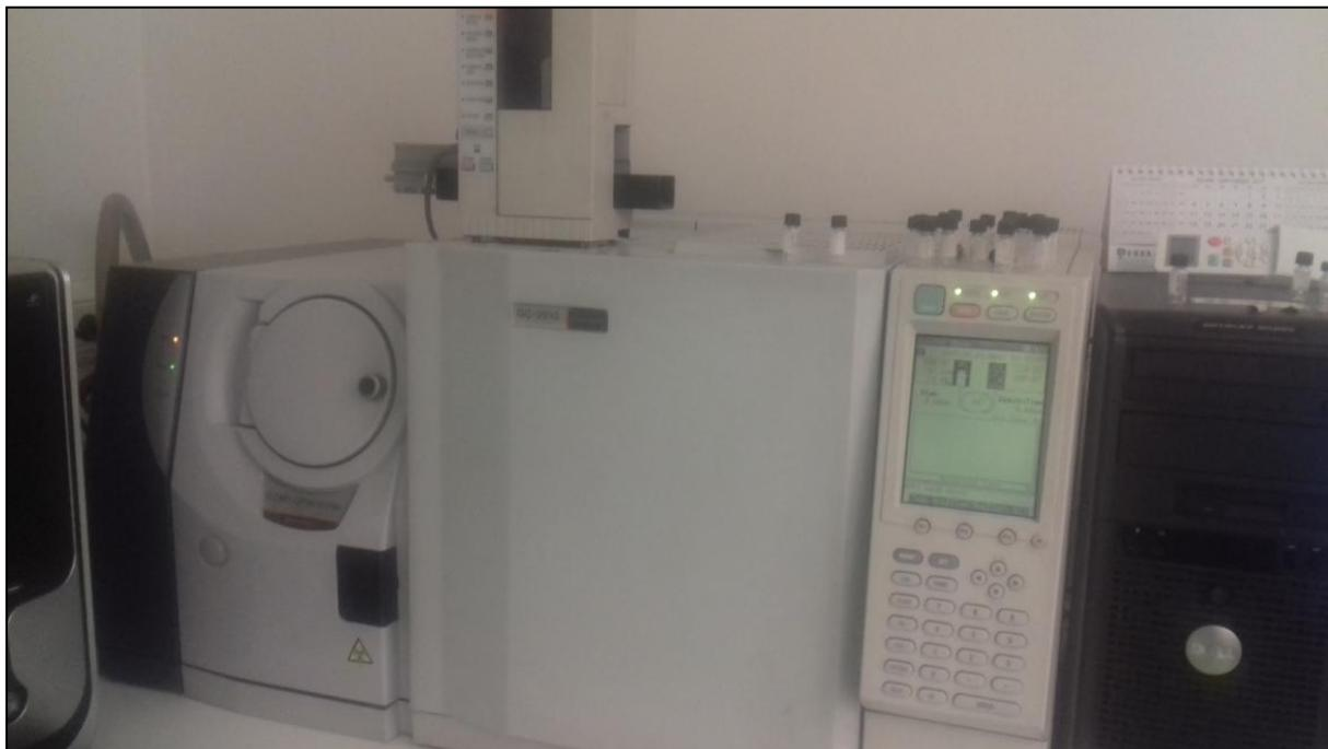
**UREĐAJ:** GC/MS (plinski kromatograf/spektrometar masa)
