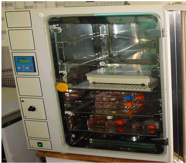
**UREĐAJ:** CO<sub>2</sub> Inkubator
